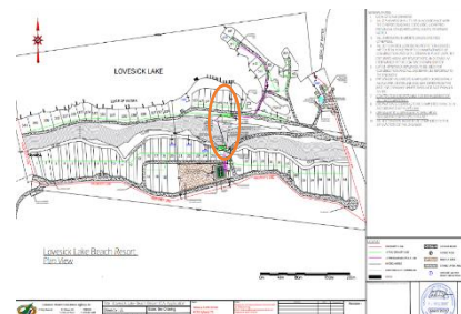
Image F – Site Plan illustrating the servicing footprint, which appears to include grading/fill placement within the erosion hazard, e.g., installing pressurized polylines, based on the ‘notes’ and ‘legends’ within the figures (ECA Design Brief).
