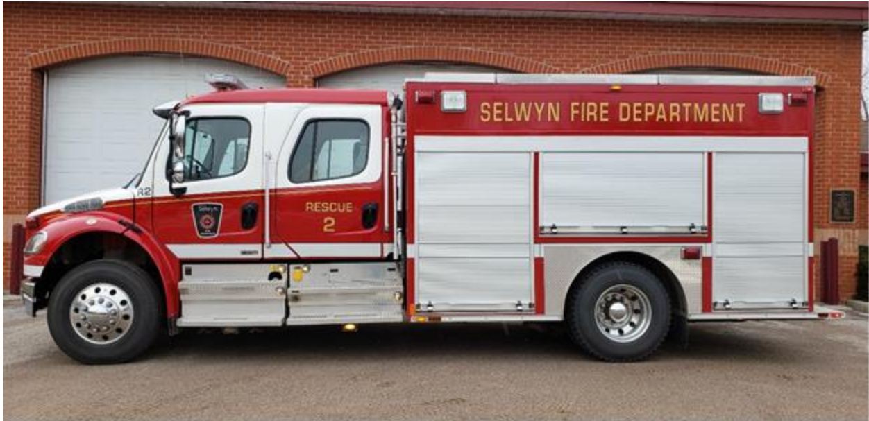
2010 - Freightliner M2-106 Heavy Rescue, 14 ft walk around box Cummins ISC 315 hp engine Allison World 3000 EVS transmission, Seating for 5
