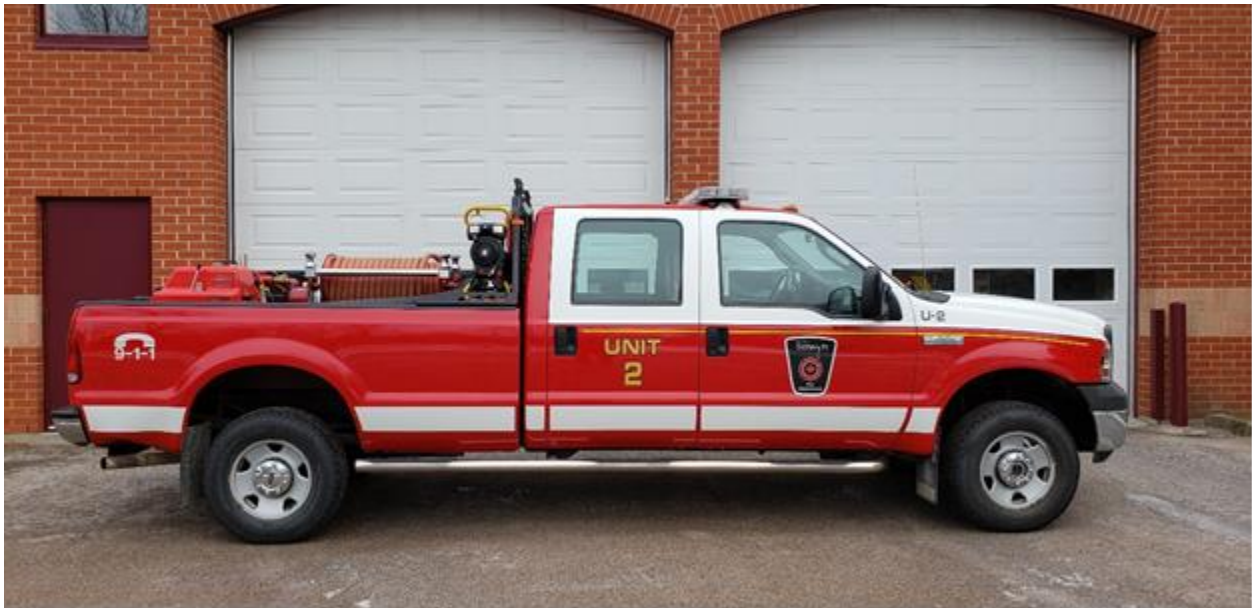
2004 – Ford F350 4X4 Crew Cab, Grass/Bush Fire Unit. 125 gal slidein Attack-Pac tank, 55hp Rabbit pump
