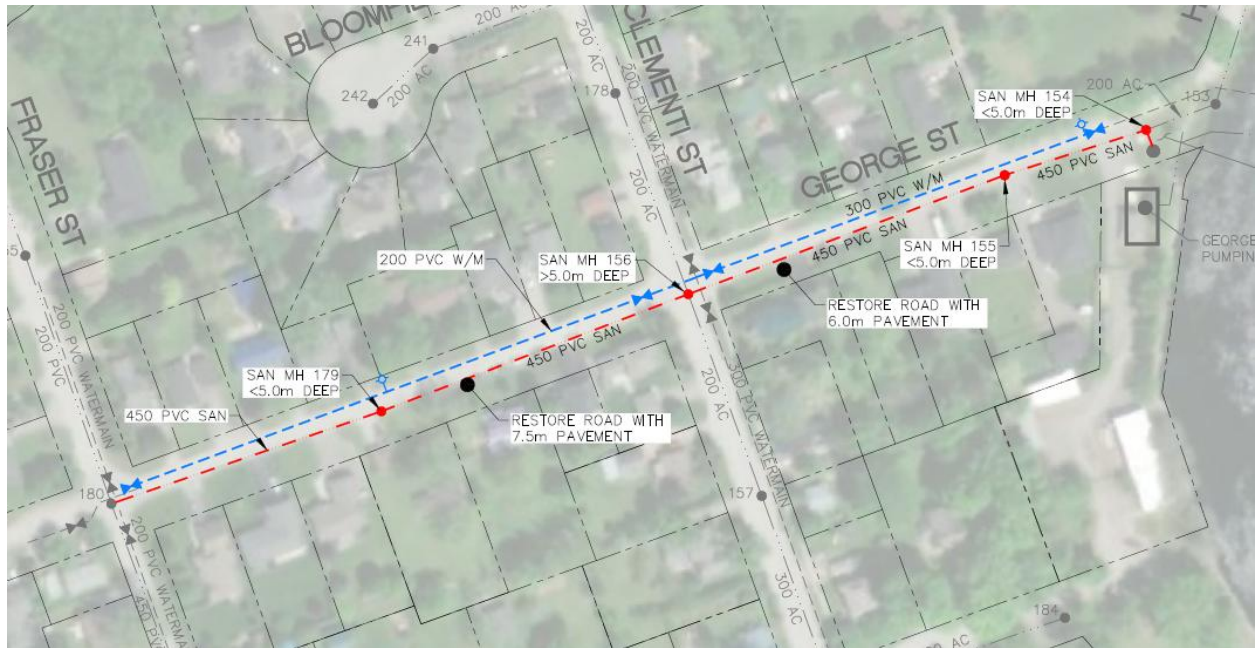
Conceptual drawing of path of George Street watermain upgrade shown in blue
