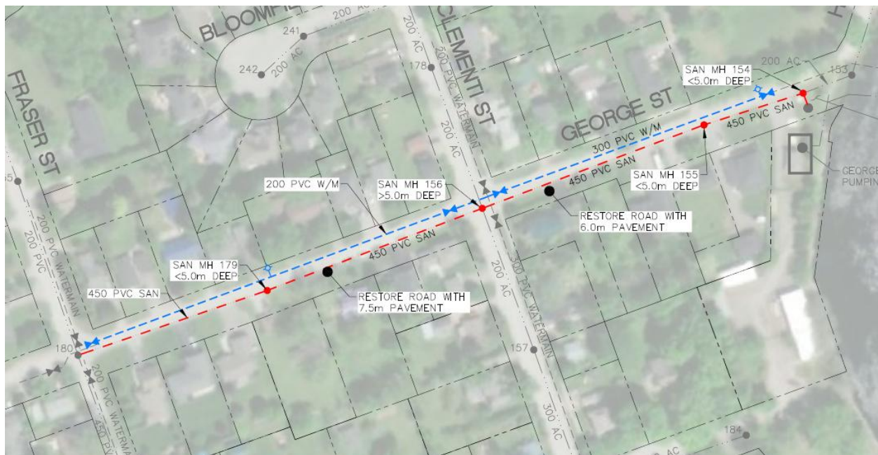
George Street Sanitary Sewer conceptual design in red
